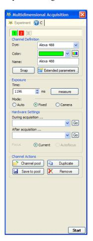
Under the C tab, you can adjust channel settings.
