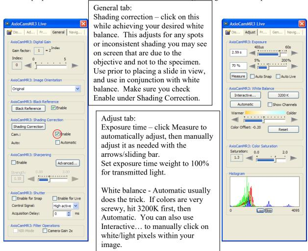
Remember to reset these three settings – exposure time, white balance, and shading correction – each time you change objectives if you plan to take a picture with that objective. Perform the latter two with no slide in place.
