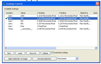
A green check mark appears next to the objective that the software believes was used when capturing the active image. If this is incorrect, select the proper objective and click "Apply selection to image."
